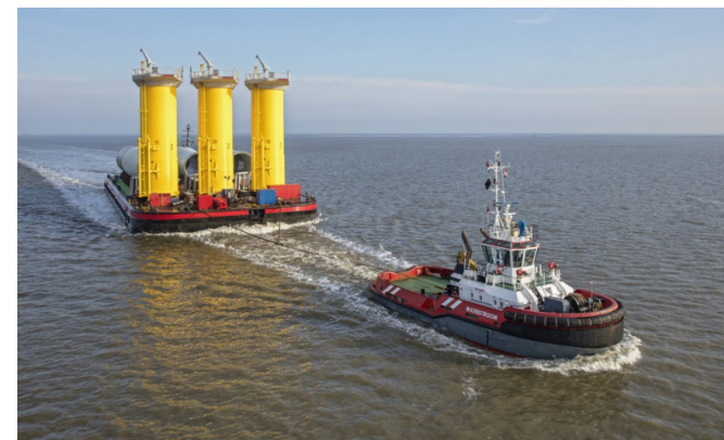
Transport of MPs and TPs to Field on Cargo Barge with single Tug
